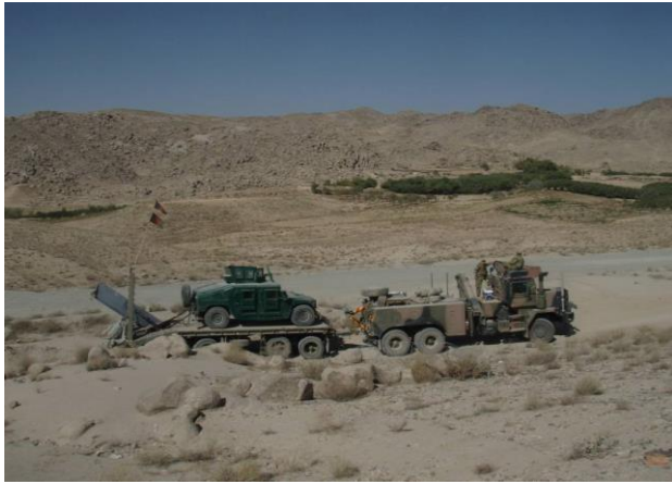
Wrecker driven by Sergeant Dave Rose and Craftsman Nathan Crosley recovers an Afghan Police Hum Vee.
