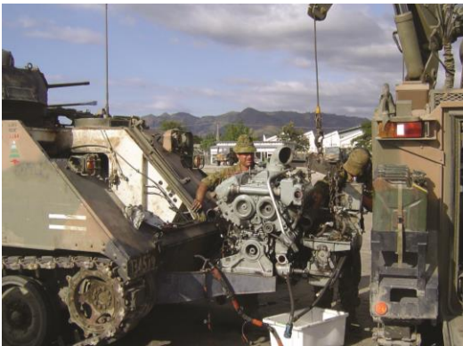
New power pack has arrived and is about to be installed.
