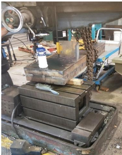
Drilling the mounting holes on the counter balance
