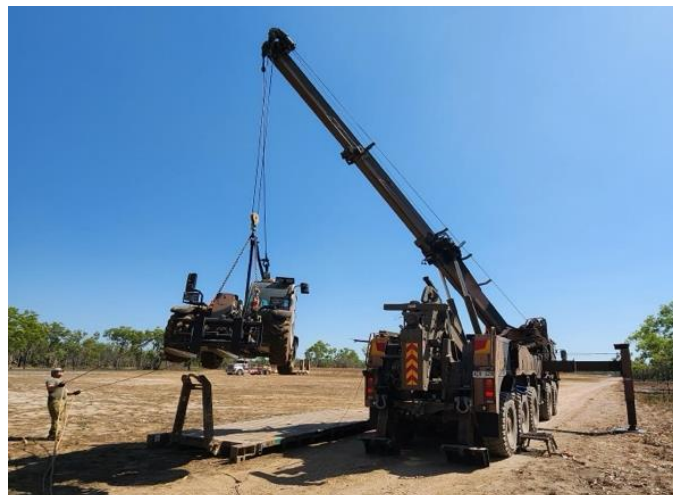
HRV lifting an all-terrain forklift onto a flat track to enable self-recovery
