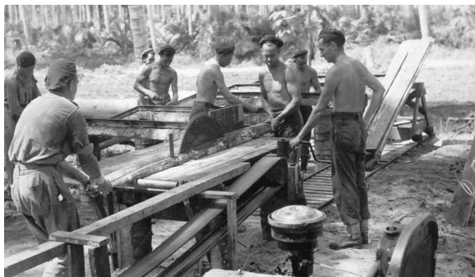
Milling coconut tree trunks with a circular saw powered by a captured Japanese engine
