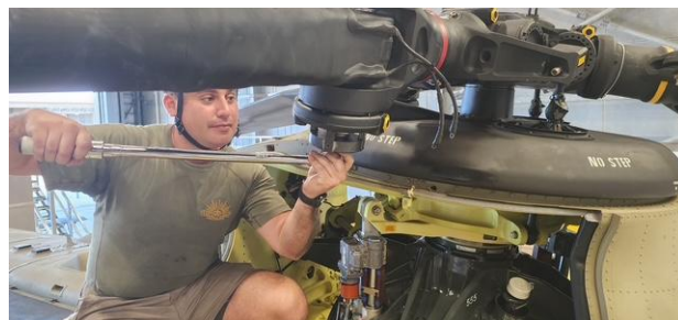
CFN B. Carrasco Undurrango torquing the lower Vertical Hinge Pin nut RAEME Association Queensland Inc
