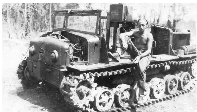
The Japanese/German Prime Mover used to pull Jeep Trains on Bougainville. The employment of this tractor resulted in the stretching of many Jeep chassis, and as a result additional work for AEME
